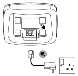
Remove the battery cover from the back of the handset and insert the 2 x AAA NiMH
